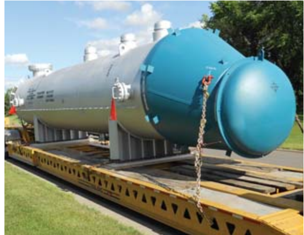
Hydrogen plant process gas boiler.
